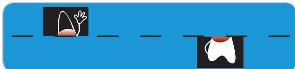
Figure 4 Tearing artifact seen when copying Frame 2 onto the screen while the vertical refresh (whose position is indicated by the dashed line) is in the same area being updated
